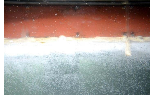
The change of the flow state along the downstream direction
