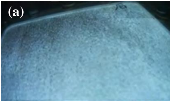
Picture of flow condition on the plate (a) Bubble; (b) Transition; (c) Air layer
