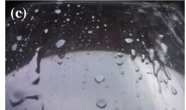
Picture of flow condition on the plate (a) Bubble; (b) Transition; (c) Air layer
